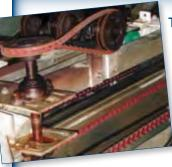
The unique link design of Classical and SP rated HPC V-Belts allows designers considerable freedom in their choice of optimum drive configuration with savings in component
