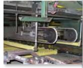
**Solution** By replacing their current belts with PowerTwist Bridge Top, the manufacturer was able to reap
